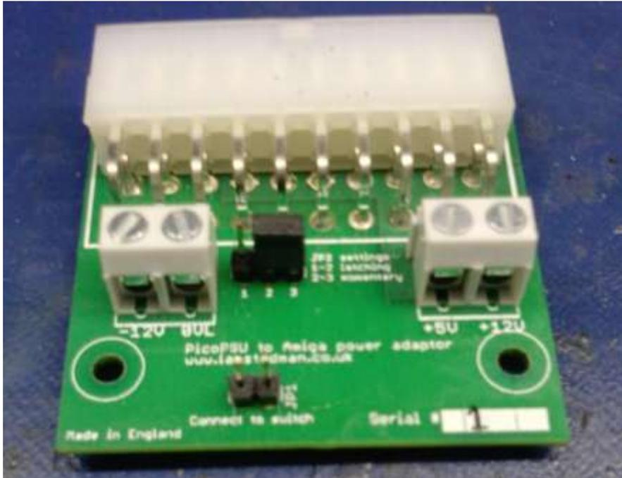
**Figure 5 Adaptor board with close up of connection detail**
