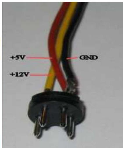
**Figure 4 CD32 PSU pinout**
