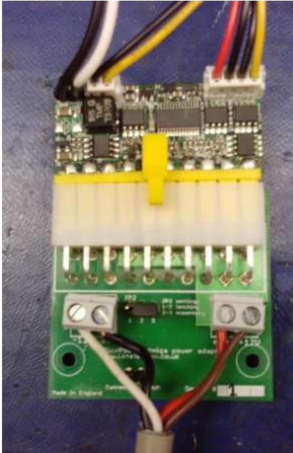
**Figure 7 Unit connected to the ATX power supply**
